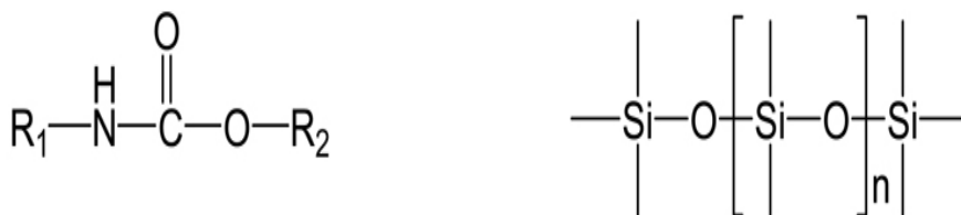
Figure 1. Chemical structures of "non-biodegradable" polymers used for drug delivery. The first structure from the left is urethane links and the second structure is polydimethylsiloxane.
