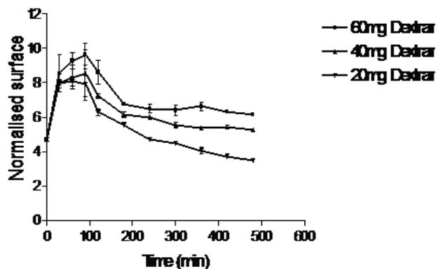
Figure 4. Surface changes of the tablets during hydration. Each point represents the mean value of the three samples and error bars show  $\pm$  S.D.
