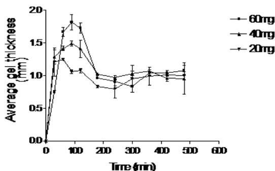
Figure 5. Gel thickness increase versus time. Each point represents the mean value of the three samples and error bars show  $\pm$  S.D.
