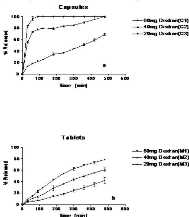
Figure 1. Dissolution profiles of capsules and tablets. Each point represents the mean value of the three samples and error bars show  $\pm$  S.D.
