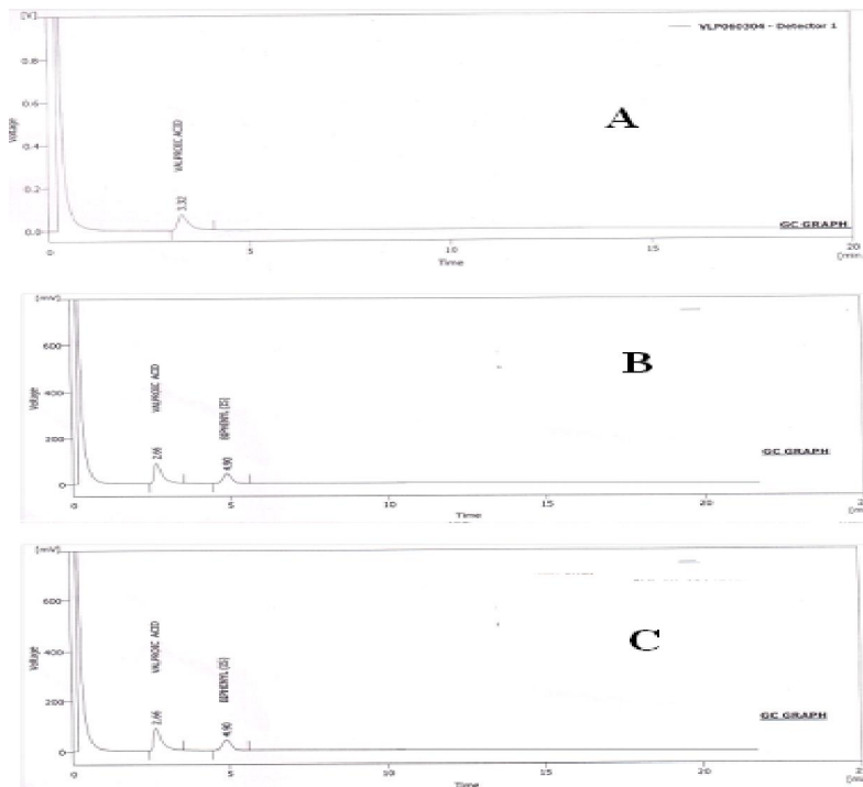
Figure 1. Gas chromatogram of (A) Standard Valproic acid, (B) Valproic acid:AEROSIL® 300 Pharma (C) Valproic acid:AEROPERL® 300 Pharma colloidal silica solid system
