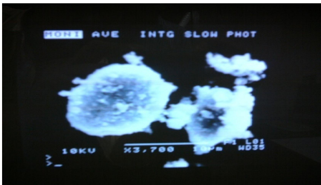
Figure 2. Scanning Electron Micrograph of Starch-Silica coprecipitate
